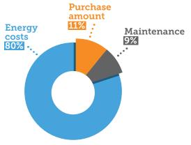
Total life cycle of a 40 bar Pet compressor calculated on a 10 year operation.
